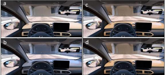
Figure 5. 4K Images of different materials used at the dashboard (a. wool, b. wool&cotton, c. bamboo, d. bamboo&cottone)
