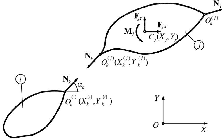
Figure 2. Isolation item with serial number  $j$ , with clearance joint.
