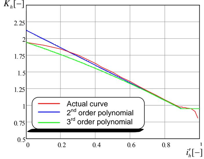
Figure 4 Torque transformation ratio modelling
