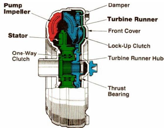
Figure 1 Torque converter components
