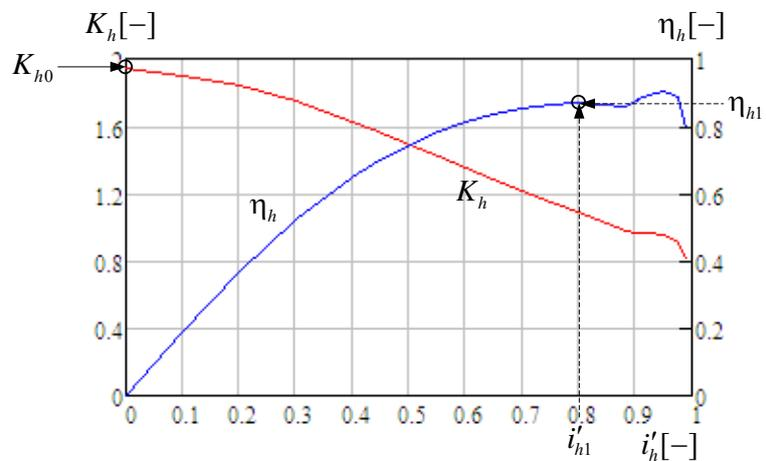
Figure 2 Typical torque converter dimensionless characteristics
