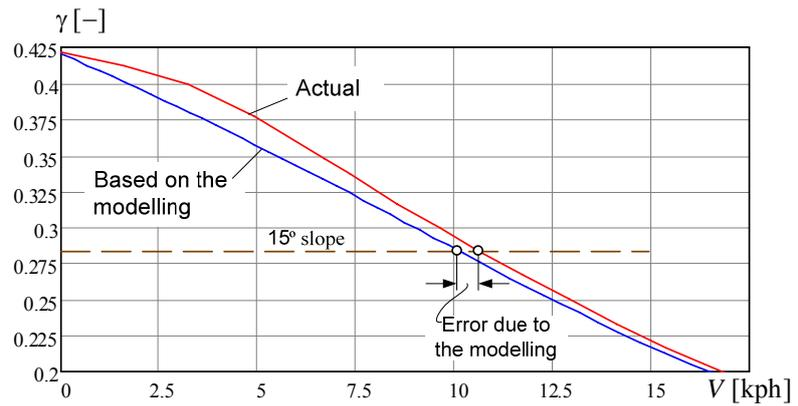
Figure 8 Detail for emphasising the error in the estimation of the speed for climbing 15° slope
