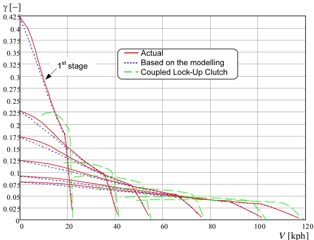
Figure 7 Tractive coefficient characteristics
