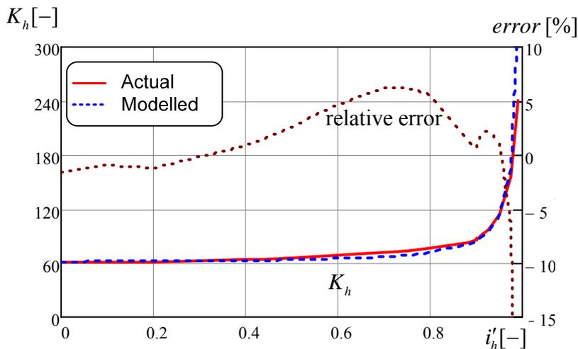
Figure 6 The absorption characteristic of the torque converter
