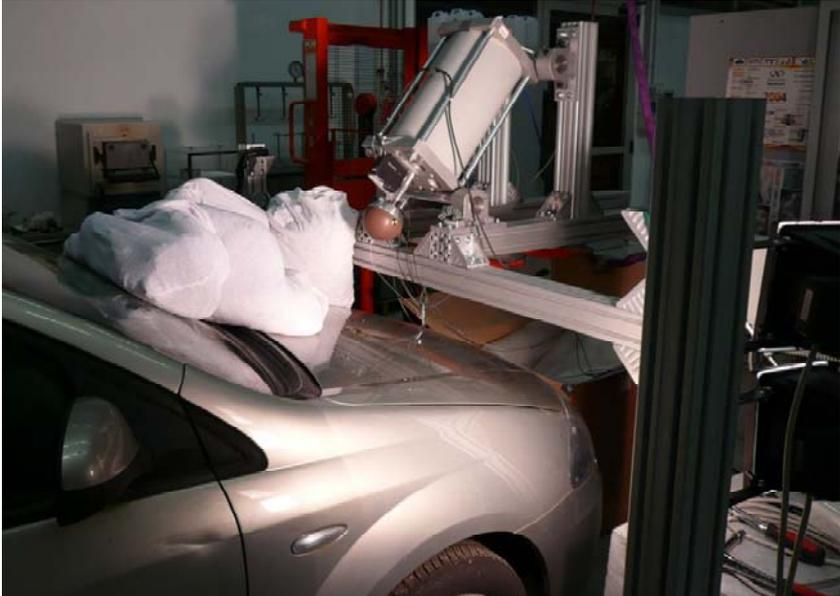
**Figure 5.** Experimental equipment for the pedestrian head impact tests
