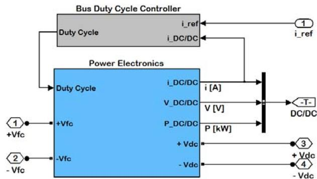
Figure 7. DC/DC converter
