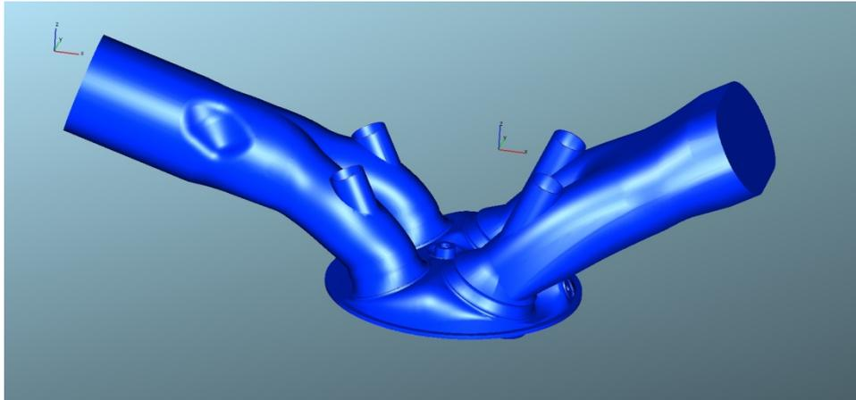
**Figure 6.** 3D geometrical model of the SCRE engine.
