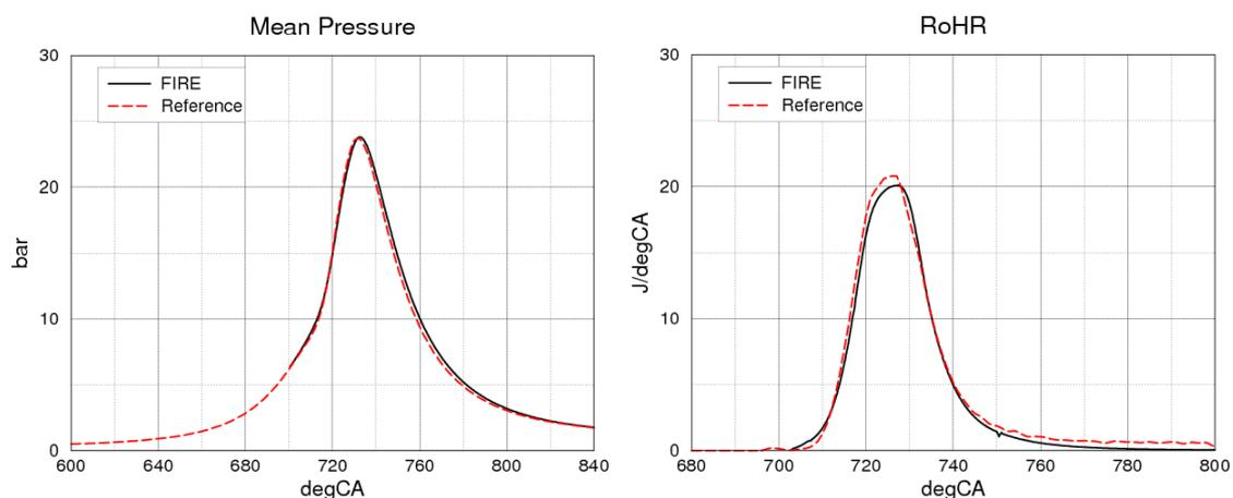
**Figure 8.** SCRE SI – Pressure and Rate of Heat Release – 2000 rpm / 3 bar, Gasoline
