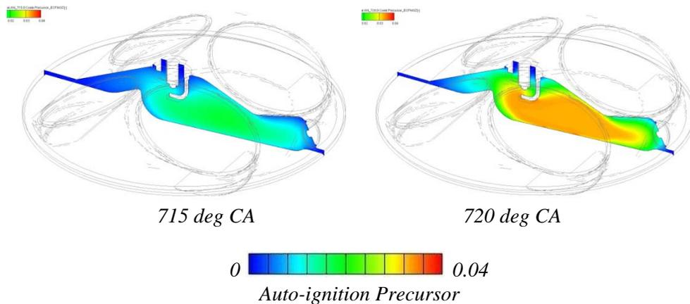
**Figure 11.** SCRE CAI – Auto-ignition Precursor – 2000 rpm / 3 bar, E85
