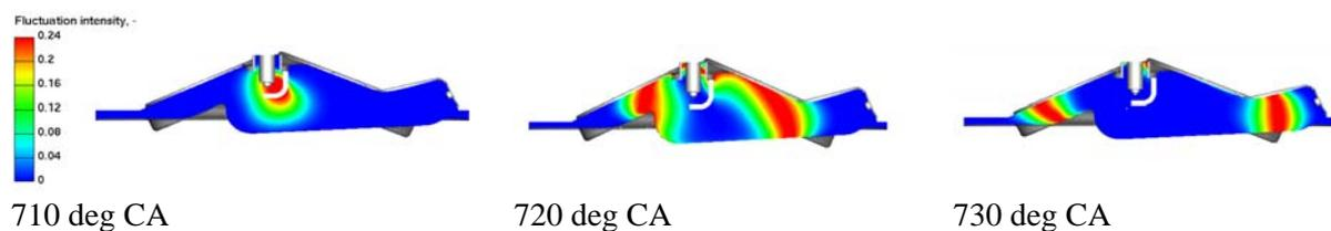
**Figure 9.** Flame front represented by the ‘fluctuation intensity’ - 2000 rpm / 3 bar, Gasoline
