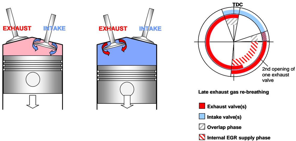
**Figure 4.** Control of Residual Gas Content for CAI Operation
