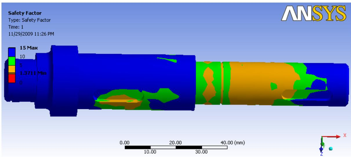
Fig. 5. Safety factor (maximum equivalent stress failure theory)
