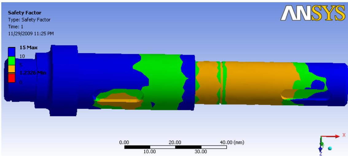
Fig. 7. Safety factor (maximum shear stress failure theory)
