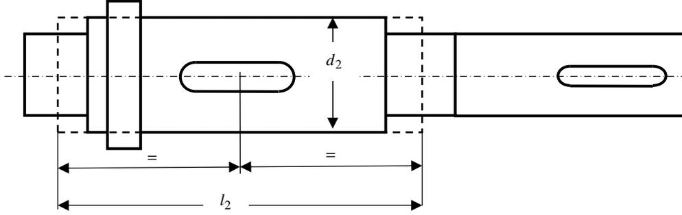
**Fig. 3. Output shaft of speed reducer**
