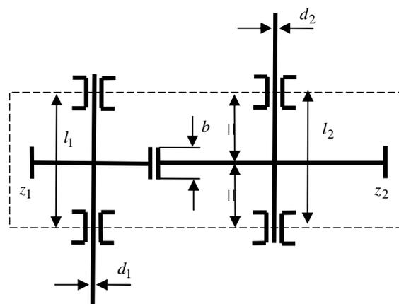
Fig. 1. A single stage spur-gear transmission
