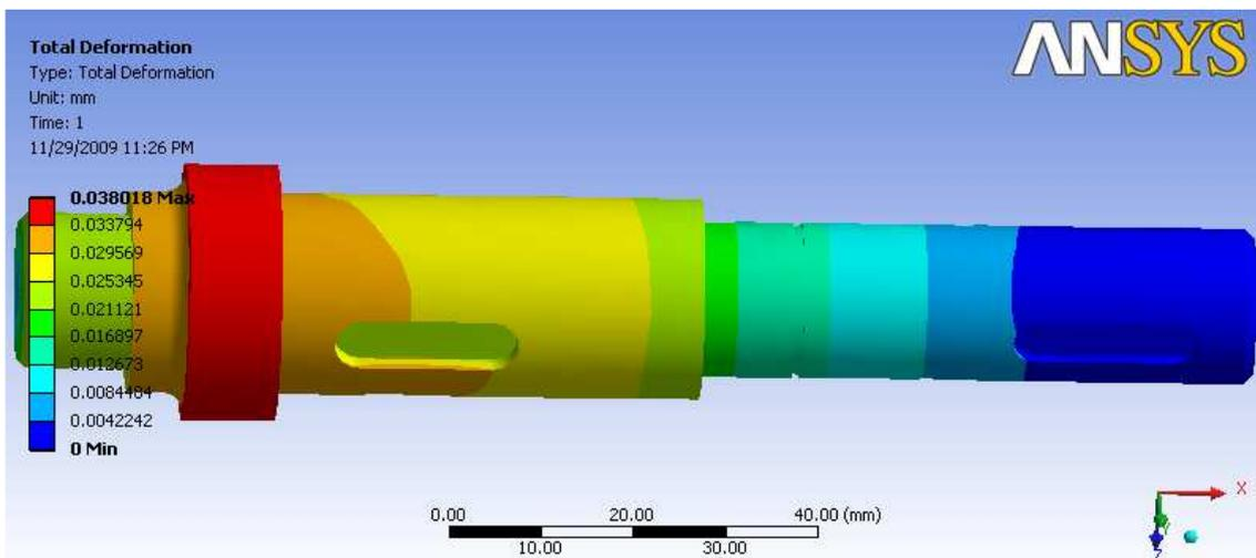
Fig. 8. Total deformation
