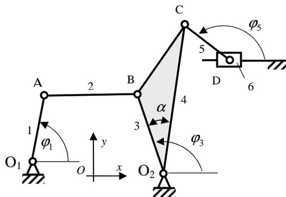
Fig. 1. Planar six-bar mechanism
