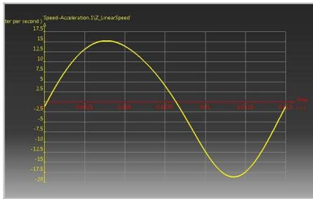
**Fig. 4.5.** PSA piston speed evolution,  $\varepsilon_v=14$ ,  $n = 4000$  rpm
