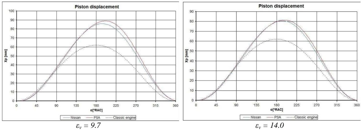
Fig. 3.2. The variation of piston displacement
