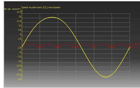
**Fig. 4.6.** Nissan piston speed evolution,  $\varepsilon_v=14$ ,  $n = 4000$  rpm
