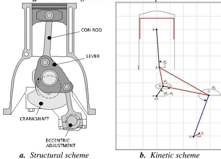
**Fig. 2.2.** Nissan engine with variable compression ratio
