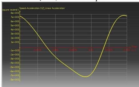
**Fig. 4.7.** PSA piston acceleration evolution,  $\varepsilon_v=14$ ,  $n = 4000$  rot/min
