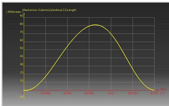
**Fig. 4.3.** PSA piston displacement evolution,  $\epsilon_v=14$ ,  $n = 4000$  rpm
