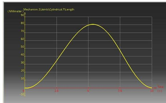
**Fig. 4.4.** Nissan piston displacement evolution,  $\epsilon_v=14$ ,  $n = 4000$  rpm
