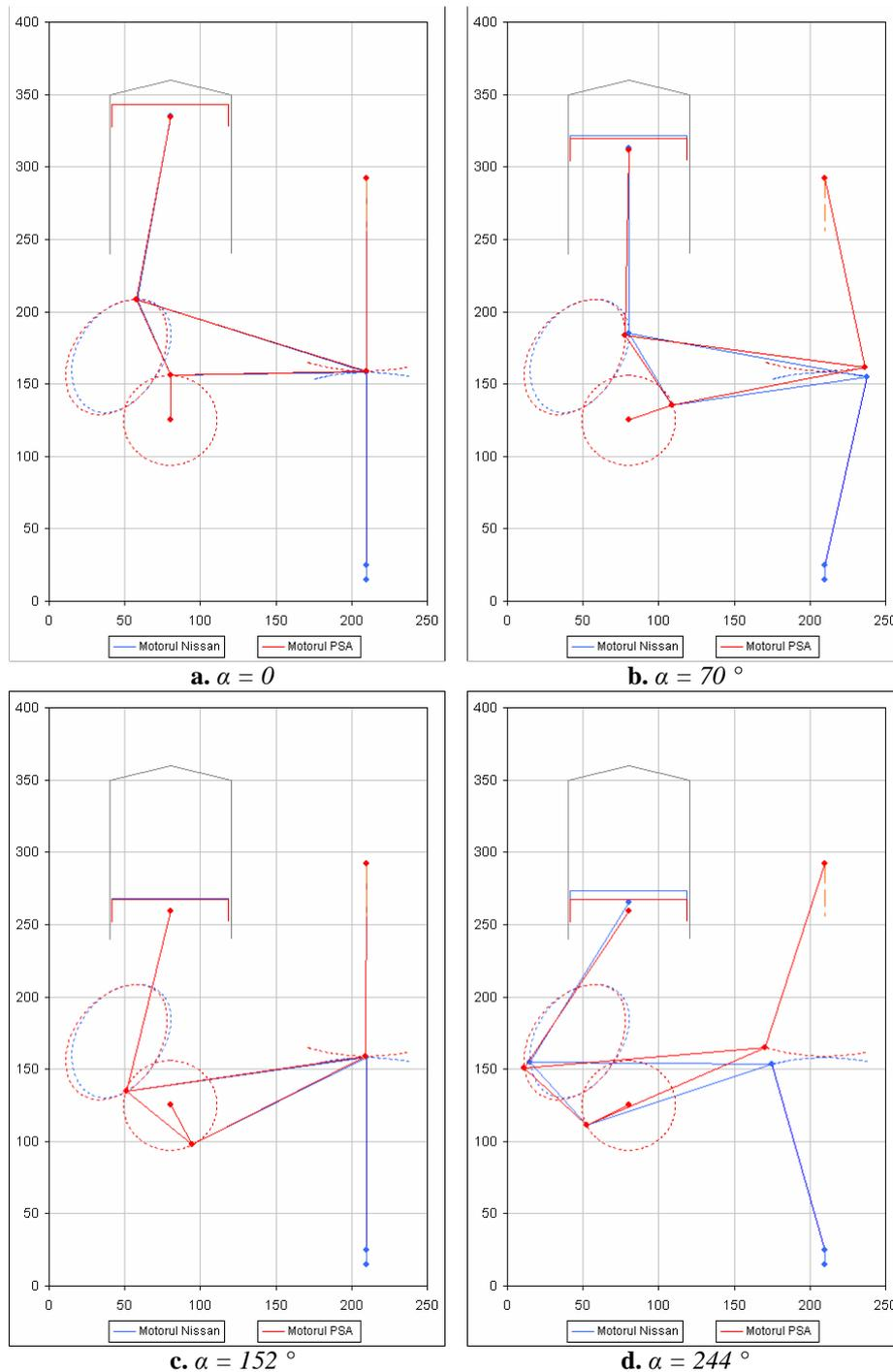
**Fig. 3.1. Superposition of the two mechanisms, for  $\epsilon_v = 9.7$**
