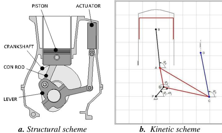
**Fig. 2.1.** PSA engine with variable compression ratio
