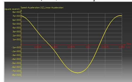
**Fig. 4.8.** Nissan piston acceleration evolution,  $\varepsilon_v=14$ ,  $n = 4000$  rot/min
