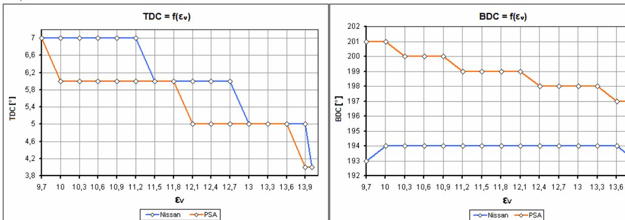
**Fig. 3.5.** The variation of TDC and BDC with compression ratio for Nissan and PSA engines
