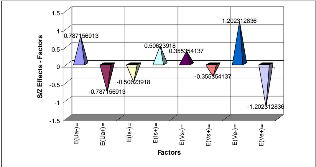
*Fig.1 The adjusted technological parameters effect ( $U_a$ ,  $I_s$ ,  $v_s$  și  $v_e$ ) on the signal/ noise ratio For the welding belt shape coefficient  $\psi$*
