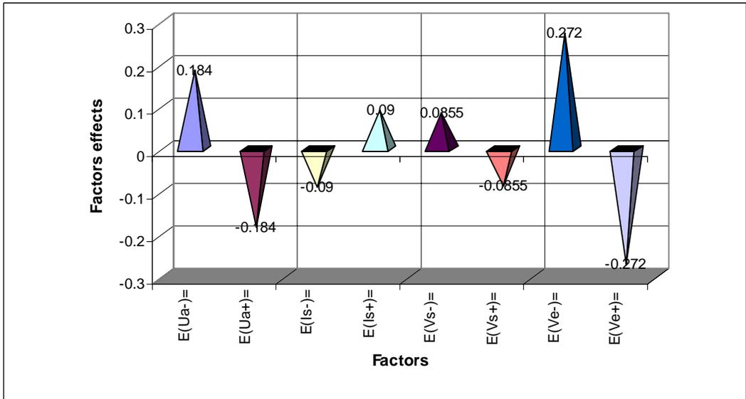
*Fig.2 the adjusted technological parameters effects ( $U_a$ ,  $I_s$ ,  $v_s$  și  $v_e$ ) on the measured Sizes for the welding belt shape coefficient  $\psi$*
