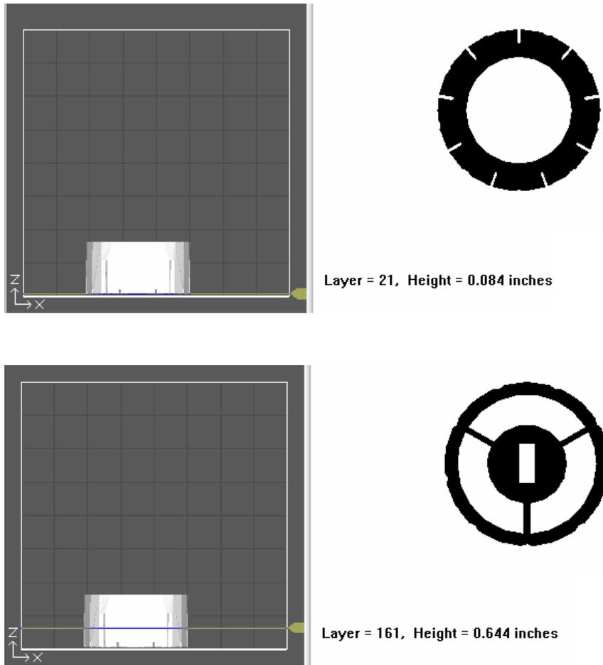
**Fig. 4. Example of cross sections on the virtual model**
