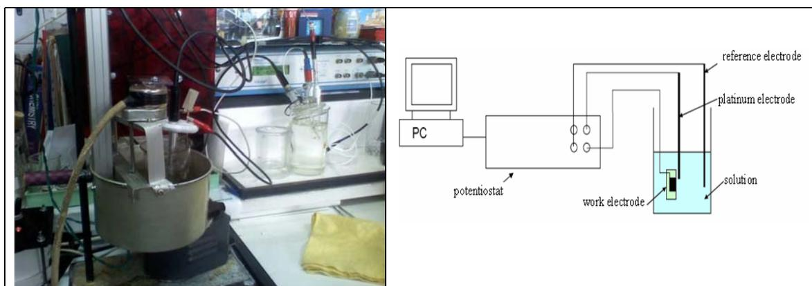
**Fig. 2 Electrochemical cell used for deposition**
