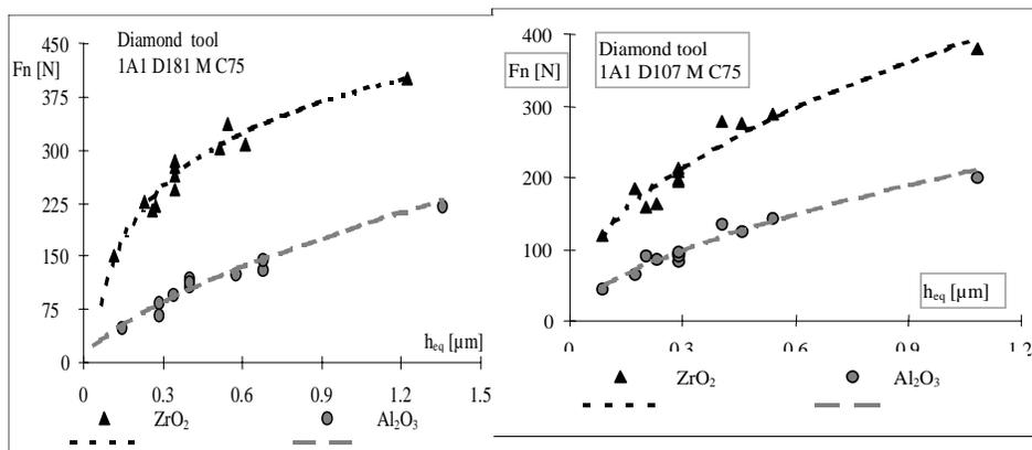
**Fig. 3 The variation of the conventional constituent of the cutting force function of the h<sub>eq</sub>**
