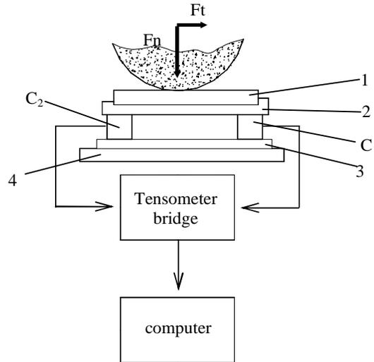
**Fig. 1. Block-diagram of the mounting used for measuring the grinding force constituents**
