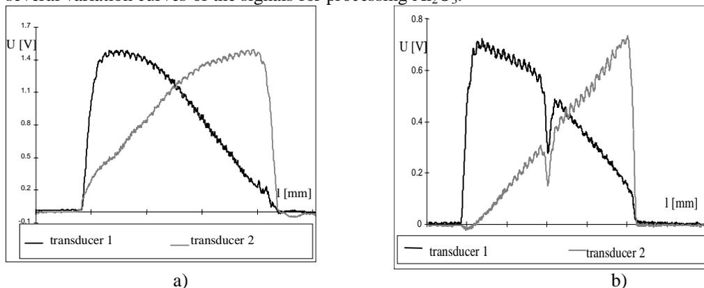
**Fig. 2. Variation of the signal given by the resistive transducers during processing a)  $ZrO_2$ ; b)  $Al_2O_3$**
