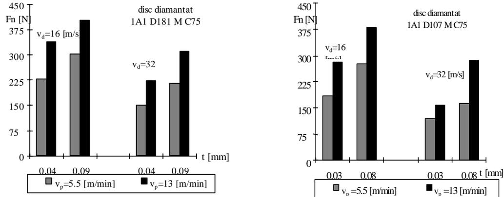
**Fig. 4. Dependency of the conventional constituent values of the cutting force to the grinding conditions ( $v_d$ ,  $v_p$  and  $t$ ), for  $ZrO_2$  processing**
