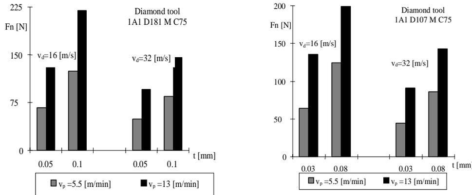
**Fig. 5. Dependency of the conventional constituent values of the cutting force to the grinding conditions parameters ( $v_d$ ,  $v_p$  and  $t$ ), for  $Al_2O_3$  processing**
